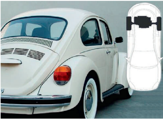
Figure 1.3 Rear-engine, rear-wheel drive
